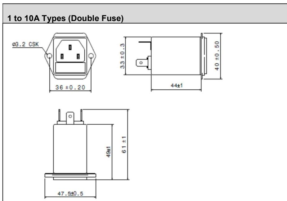
All dimensions in mm; Tolerances according to ISO2768-m
